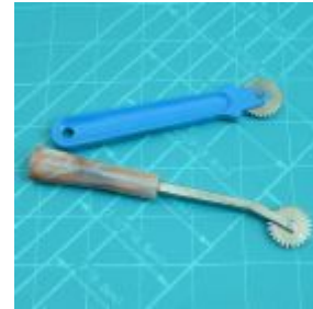
Tracing Wheel — Wheel used along with tracing paper to transfer sewing details to fabric
